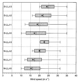
FIG. 11. Distribution of wind speed maxima for the southerly and northerly LLJ categories. Shown for each category are the minimum (left whisker), the maximum (right whisker), the median (dots), the mean, the mean plus one standard deviation, and the mean minus one standard deviation (vertical lines in the shaded box).
