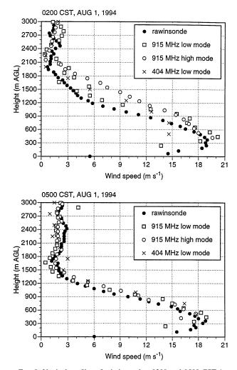
FIG. 8. Vertical profiles of wind speed at 0200 and 0500 CST 1 August 1994.
