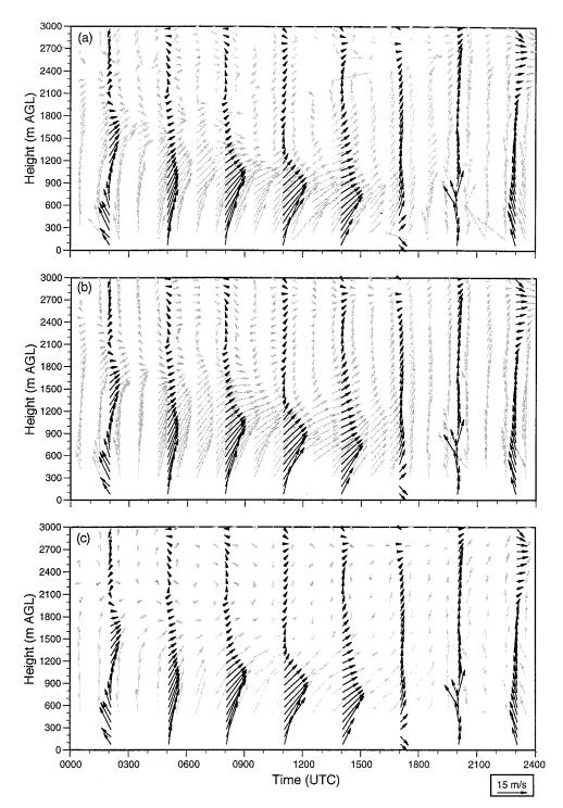
FIG. 7. Comparison of rawinsonde vector wind profiles (dark vectors), averaged over 100-m height intervals, with those measured (gray vectors) by (a) the low mode of the 915-MHz wind profiler, (b) the high mode of the 915-MHz wind profiler, and (c) the 404-MHz wind profiler for a 24-h period starting at 1800 CST 31 July 1994.
