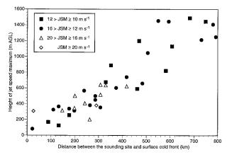
FIG. 18. The height of the jet speed maxima (JSM) for northerly LLJs as a function of distance behind the surface cold front.
