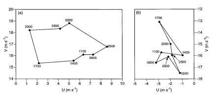
FIG. 14. Diurnal oscillations of wind speed and direction at the maximum jet wind level for (a) southerly and (b) northerly LLJs. The U represents the eastward wind speed component and V the northward component. Indicated times are central standard time.
